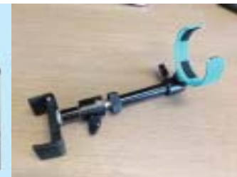
Figure9. (right) showing Mechanical prototype of lens-to-smartphone mount with 3D printed Panretinal 2.2 condensing lens holder
